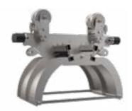
Trolleys made of AlSI304/316 stainless steel, and stainless steel mechanical fasteners. Designed to travel on IPS 180 type profiles, having 4 x  $\emptyset$ 120 Zinc plated steel wheels and 8mm thick polyurethane covering. This covering allows the design to be classified as Explosion-Proof. They also have side and bottom rollers to prevent bouncing and excessive drift.
