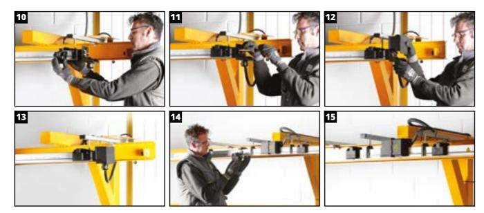
Introduce in the end of the line, or using any housing joint, the collector trolley, by manually pressing the brushes, taking into account it only has one position: The brush marked as "Earth" has to be located on the side of the PVC profile indicated with black and white stripes, and with an "RG" sticker (Photo 16).
