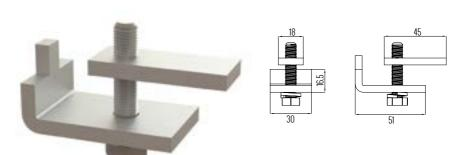
System component SUMM-500. Made from threaded plate, curved plate, M10 bolt and grover washer, Galvanized steel
