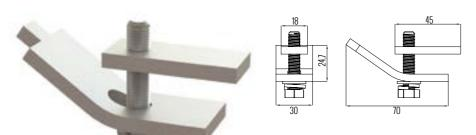
System component SUGMM-500. Made from threaded plate, curved plate, M8 bolt and grover washe. Galvanized steel.
