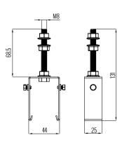
Manufactured from steel sheet with blue Epoxy paint finish RAL 5010.
